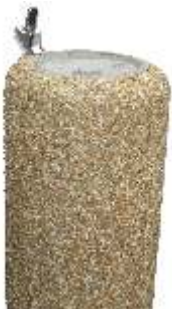
CIVIC DRINKING FOUNTAIN MK1 and MK2 1200mm overall (also Child Step available). Approx 850mm above ground. 320mm diam. For MK2 take a 610mm tree ring to form a pebble base water soak-away.
