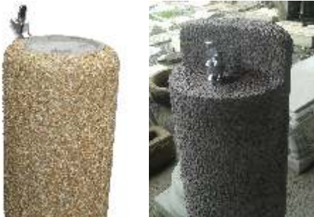
CIVIC DRINKING FOUNTAIN MK1 and MK2 1200mm overall (also Child Step available). Approx 850mm above ground. 320mm diam. For MK2 take a 610mm tree ring to form a pebble base water soak-away. Do not lift by tap - it will break.
