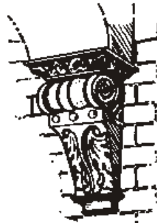
LEAF CORBEL 475mm high Cap 134 x 265 x 75mm high Cap is loose.
