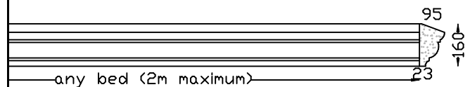
WB VENEER LINTEL Max 2,000m bed. Larger sizes in more than one piece.
