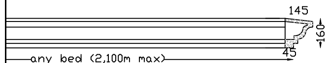
WOODLANDS VENEER LINTEL FRC Max 2,100m bed. Larger sizes in more than one piece.
