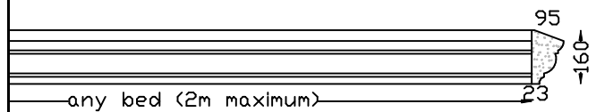
WB VENEER LINTEL Max 2,000m bed. Larger sizes in more than one piece.
