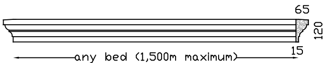
HAMPTON 120 VENEER LINTEL Max 1,600m bed. Larger sizes in more than one piece.
