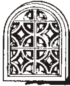
CLOISTER GRILLE 724 x 572 x 100mm
