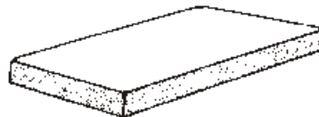
SMOOTH CAST, REINFORCED 910 x 330 x 50mm 910 x 330 x 75mm 910 x 240 x 75mm 760 x 200 x 50mm
